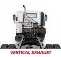
For custom body mounting and special equipment, exhaust is relocated from the frame rail to directly behind the cab. Available on N-Series Standard Cab only.
