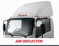
To help maximize fuel efficiency, the customdesigned Isuzu air deflector directs air over the top and around the sides of body to reduce drag.
