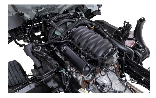
The rigorous driving demands of medium-duty trucks require a durable powertrain. Integral to this is a cast-iron block specifically designed for heavy-duty use with channels incorporated for jet-spray piston cooling to help the engine run cooler and *more efficiently*. Additionally, an aluminum head design incorporates direct injection, variable valve timing, and an air intake humidity sensor that manages the 6.6-liter
