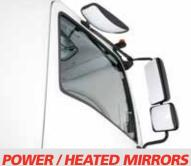
Heated flat and convex mirrors with or without dual remote controls. Heated mirrors prevent fogging and ice collection with a quick push of a cab switch. For added convenience, available remote controls allow the driver to quickly adjust the angle of the mirrors.
