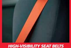
High-visibility orange seatbelts provide quick visual verification that seat belts are being worn to conform with safety regulations. (Driver and right passenger seat only.)
