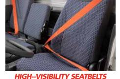
High-visibility orange seatbelts provide quick visual verification that seat belts are being worn to conform with safety regulations. (Driver and front right passenger seats only.)
