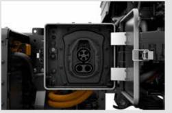
To accommodate their multiple battery packs and to provide reasonable charging times, NRR EV trucks, with battery capacities of 60, 100,140, and 180 kWh, have an AC charging time range from 5.5 to 10 hours and a DC charging time range from 1 to 2.5 hours.
