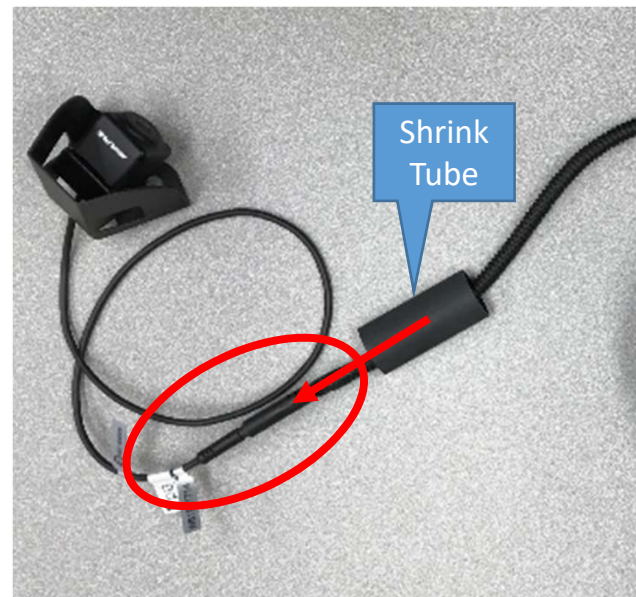
Figure 66 Camera Install Kit Shrink Tube Installation
