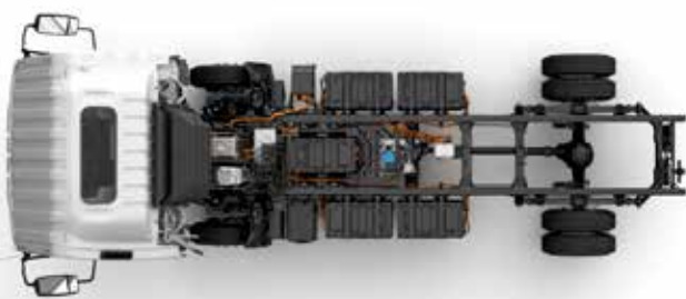
5 Battery Packs - 100 kWh
